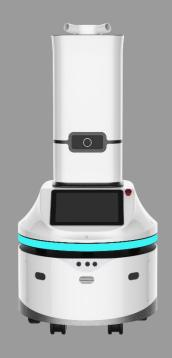
Powered by an internal disinfection system, the smart robot can take over extensive floor and air disinfection at hospitals, offices, factories, schools and other public facilities. It operates on auto-pilot along preset routes to accurately and efficiently spray disinfect in various work modes, and automatically returns to base for recharging at low power.
