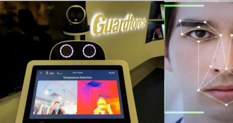
Guardforce Smart ConcieGuard combining visitor management system, concierge, customer services, access control and surveillance features has added a new function for measuring visitors' body temperatures, a perfect device to record body temperatures and prevent the spread of the virus.
